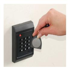
**Programming** The installer programs these items -(a) In the KP-6840, <u>keypad output format</u>, either 4bit or 8-bit key-bursts, or 26-bit code transmission (like a reader with a 26-bit card). (b) In the KP-6840 if the keypad has 26-bit output, the <u>facility code</u> that the customer requests. (c) In the system's computer, the KP-6840's <u>Operation Mode</u>.
